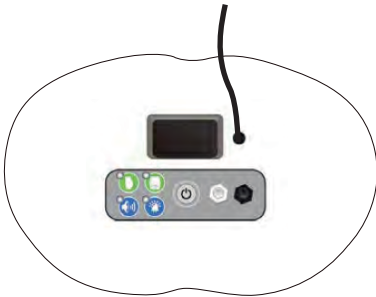
<AC Power Connection>
